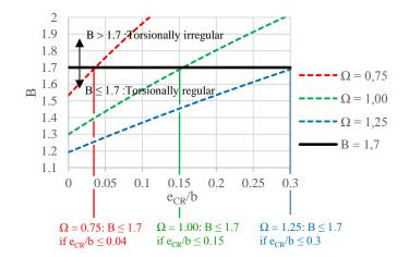
Figure 5: Torsional Irregularity Parameter B
