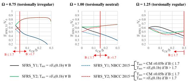
Figure 8: Comparison between SFRS element design forces obtained by the two NBCC 2015 methods for accidental torsion Montreal class C
