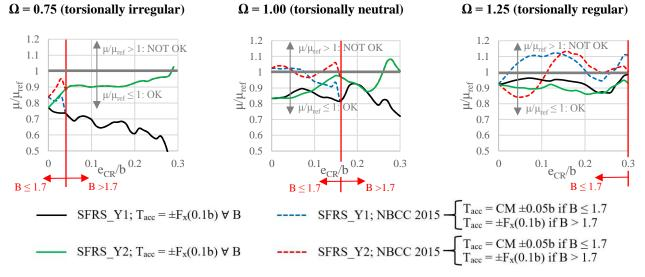
Figure 11: Normalized SFRS ductility demands on SFRS elements designed with  $R_d = 3.0$ .
