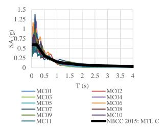
Figure 9: Spectral acceleration SA of ground motions calibrated using Montreal class C design response spectrum
