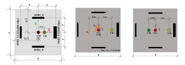
Figure 1: Plan view of the building used for parametric analysis
