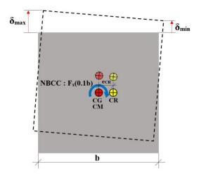
Figure 4: Building plan view illustrating parameter B calculation
