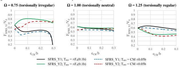
Figure 7: Comparison between normalized SFRS element design forces obtained by applying accidental torsion as a static torque to those obtained by displacing the CM for a uniform spectrum
