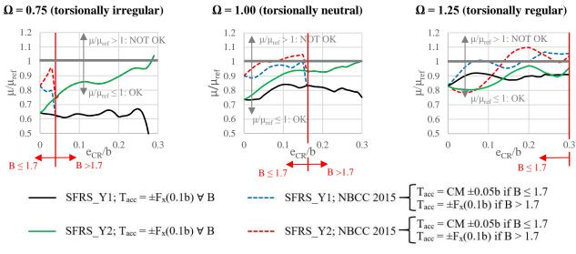
Figure 12: Normalized SFRS ductility demands on SFRS elements designed with  $R_d = 5.0$ .
